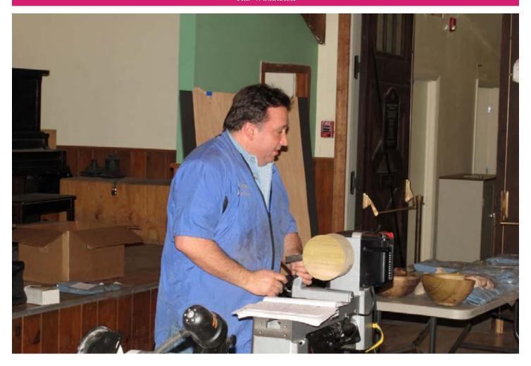
For stability, your tool handle length needs to be need 5X the overhang over the tool rest. In other words, a tool with the cutter 4" past the tool rest needs to have a 20" handle.
