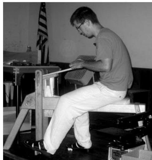
A horse such as this is perfect for holding irregularly shaped objects for the spoke-shave. Strother sharpens his blades razor sharp, but does not make new chip breakers (such as those featured in Fine Woodworking)
