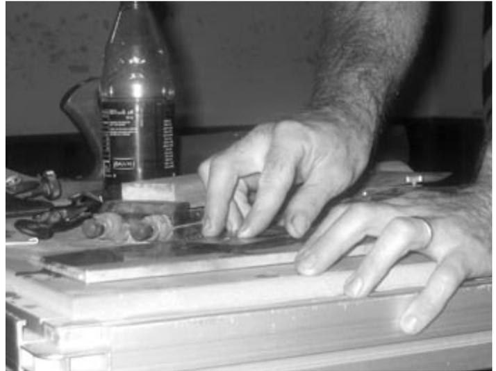
Proper hand position over the sharpening stone
