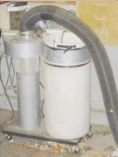
Jet 610 CFM dust collector with fine mesh filter bags.
