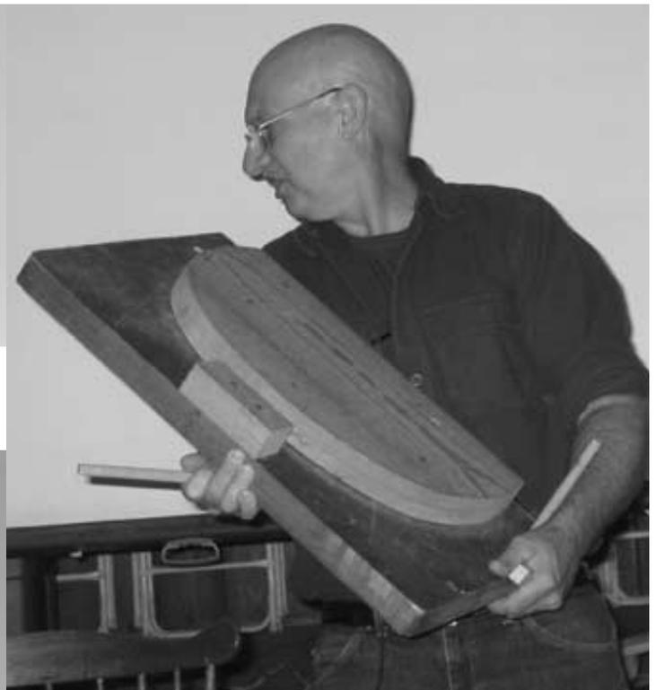
Bending jig used for steam bending the chair back. You have about 40 seconds to curve and clamp the thin wood (usually oak) material.
