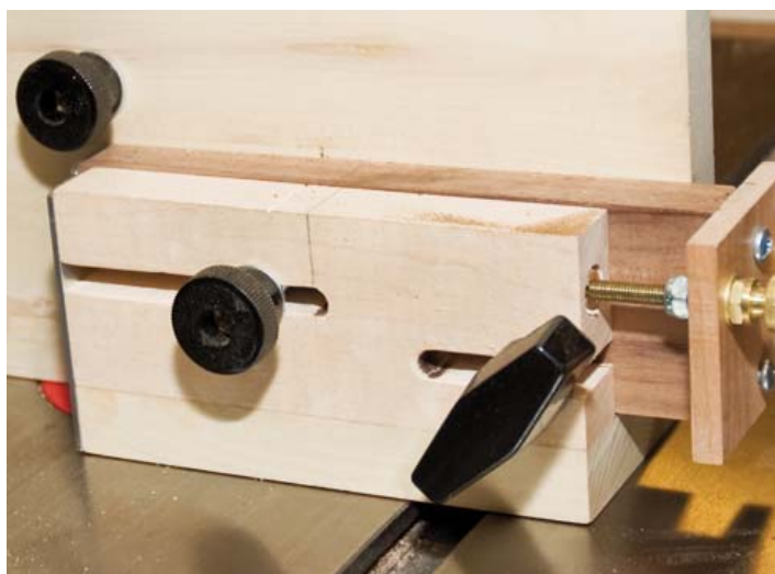
An adjustable box joint jig made by Steve. The rear of the box joint jig shows adjustable brass knobs. The near knob adjusts the width of the key and the back knob the width of the slot. The two black knobs respectively lock in the two settings.
