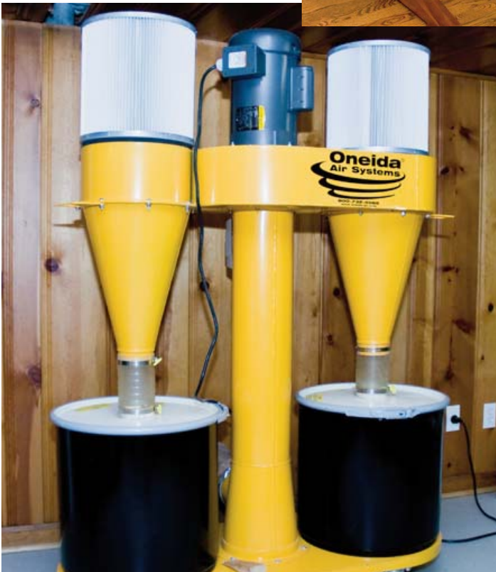
A 3 hp Cyclone dust collector keeps Steve's downstairs shop and upstairs chip and dust free.
