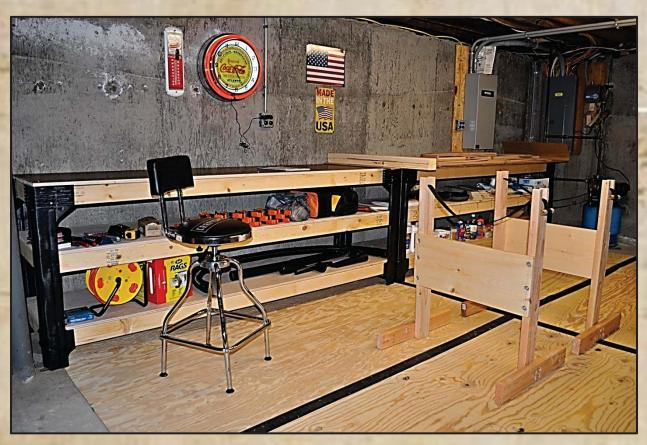
Wood floor approx. <sup>1</sup>/<sub>4</sub>" X 8' X 16'; benches total 16' length X 2' deep X 32" high. There are two work stands that can be quickly converted to sawhorses. The near bench holds a number of frequently used tools. The picture shows a freshly prepared, but as yet unused workshop.
