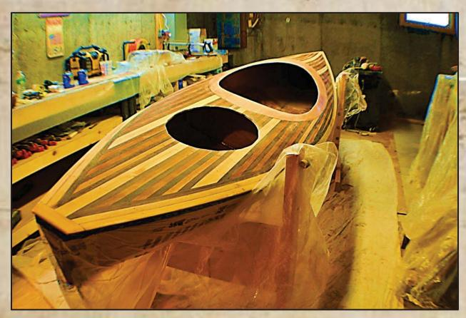
Each fiberglass application required 3 layers of epoxy to achieve a smooth surface by completely filling the weave of the cloth.
