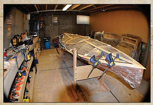
The strips needed to butt the coaming apron. Note the sharp angles that were hand-cut for the strips as well as the curves and twists they must accommodate.
