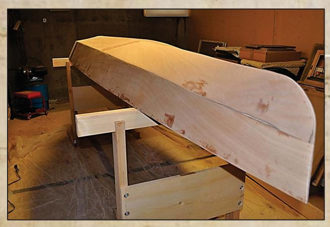
Note the (\*%\*%\*^ sand-through near the bow. The top-most layer of the ply is about 1mm thick or about 0.04". Need to think up something clever to cure the boo-boo... The stands are in their sawhorse configuration.
