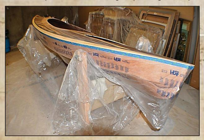
Thank goodness for tape and plastic sheeting! The initial epoxy application to glass the deck resulted in many hours of sanding to remove drips and to "feather" in the fiberglass along the side panels.
