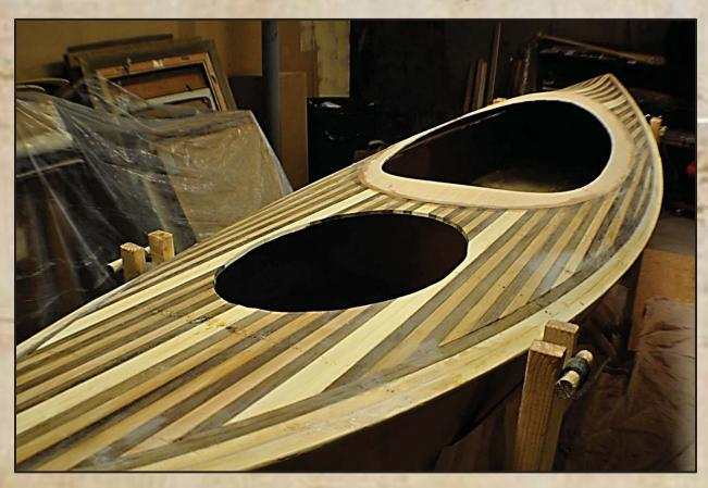
Staple marks were clearly visible. Rather than using staple-less techniques, staples were used to ensure the strips closely followed the forms. There are different schools of thought regarding the esthetics of marks due to staples or other fasteners which are byproducts of the construction process. Some folks like them, others not so much.
