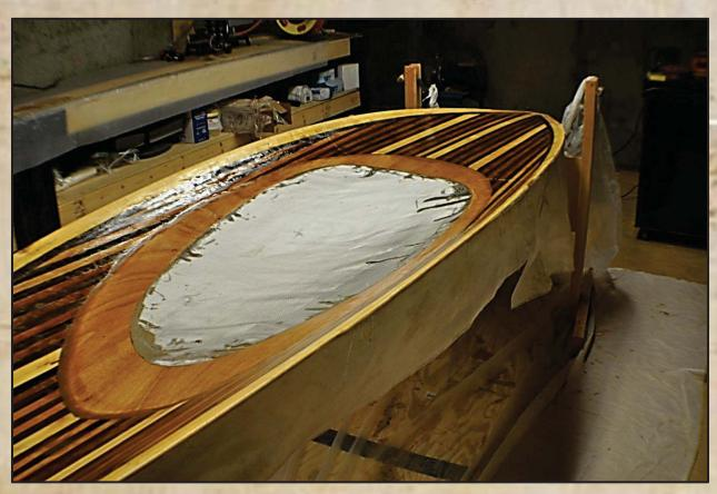
Note that the coaming apron was joined to the strips by epoxy fillet (pronounced appropriately, fill-it). The excess fiberglass had to be trimmed from the coaming apron and deck edges. Reaching this milestone required lots of sanding and multiple coats of epoxy (with more sanding between applications).
