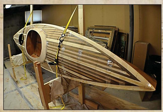
Packing tape was used to hold the deck in place temporarily. The craft was turned on its side in anticipation of epoxying 3" fiberglass tape along the full length of the side seams. After the first side was completed, the boat was turned and the other side was glassed. The forward section was particularly difficult since the cockpit-to-bow length is far longer than the builder's arm; a home-made tool described in the WDH-12 manual was used to facilitate the process.
