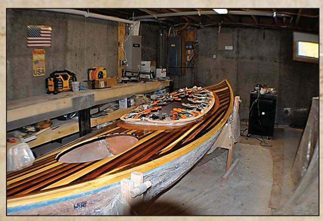
Clamps, anyone? The coaming assembly was a sandwich of 2 spacers and a top piece. The picture was taken immediately after the parts were put in place.
