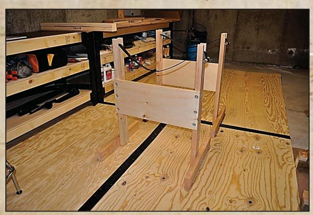
Each stand was built from a single 2" X 4" X 10' board +  $\frac{1}{2}$ " X 12" X 27" piece of pine. The straps were constructed from 1½" wide webbing and a couple of pieces of dowel, 1" X 4". This configuration held the boat right-side up.
