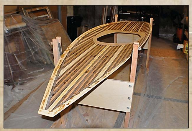
The wet spots were due to glue that had seeped through the joints. Thank goodness for the protective plastic wrap.
