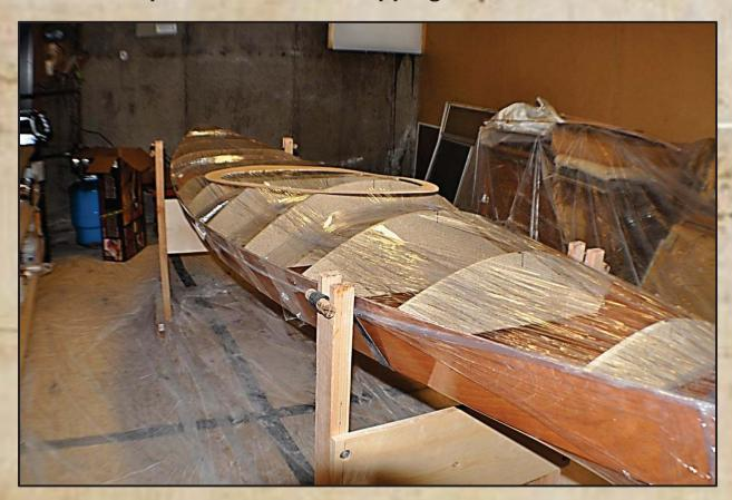
Another angle... The wooden circle-like object on the top of the hull is the coaming apron. It was positioned thus to verify fit and placement of the forms.
