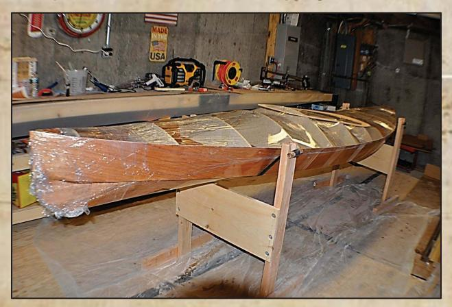
The hull was wrapped in plastic to protect the finish from rubs and glue drips during the stripping process.
