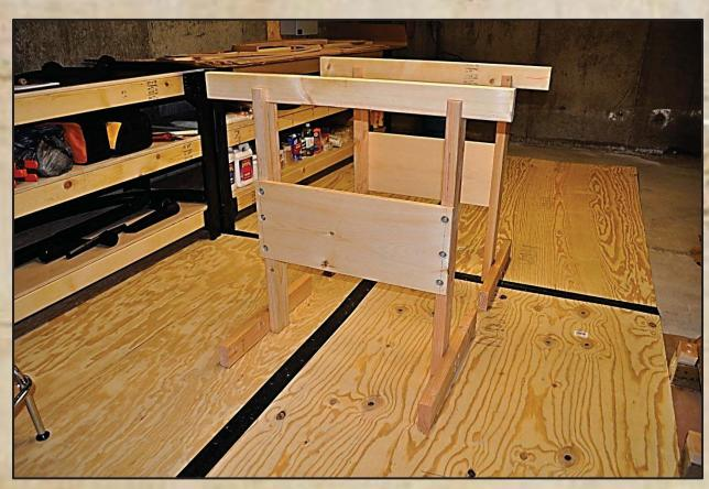
This configuration was used whenever the boat needed to be positioned upside down.
