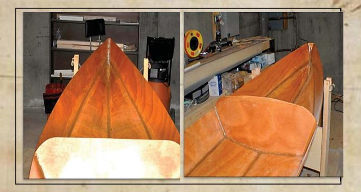
Shop-fabricated arch insert included: 2 coats of epoxy; attached with Titebond III and fillet; fiberglass; 2 more coats of epoxy.
