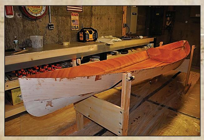
Note the copper "thread" and hull forms have been removed. The vertical piece is the bulkhead. The seams have been filleted and the inside has been fiberglassed and epoxied. Note the craft was supported by the work stands in their sling configuration.
