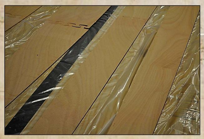
Note puzzle joints... Look carefully - the 3<sup>rd</sup> board from the left has a partially assembled puzzle joint. Before gluing the author needed to determine which board sides were cleaner, i.e. had better grain and fewer imperfections.
