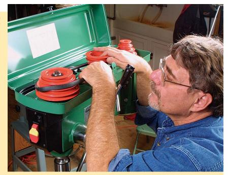
Setting belt tension. Belt tension is adjusted by moving the motor away from the spindle. All of the models have a crank handle for this adjustment.
