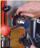
Two styles of depth locks. On the models examined, the depth lock (which sets the bit depth) is often mounted on the feed handle (above) or on a simple stop mechanism (right) with knurled nuts.
