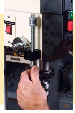
Depth lock slides into place. For easy depth adjustment. Delta's depth locknut slides up and down with the push of a button.
