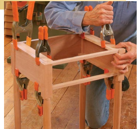
No joinery for runners, kickers, and spacers. The runners and kickers are simply glued and clamped into place (above), flush with the top and bottom of the aprons and rails. Plane the spacers perfectly flush with the inside faces of the legs before gluing them on (below).
