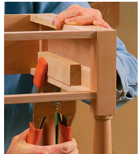
No joinery for runners, kickers, and spacers. The runners and kickers are simply glued and clamped into place (above), flush with the top and bottom of the aprons and rails. Plane the spacers perfectly flush with the inside faces of the legs before gluing them on (below).
