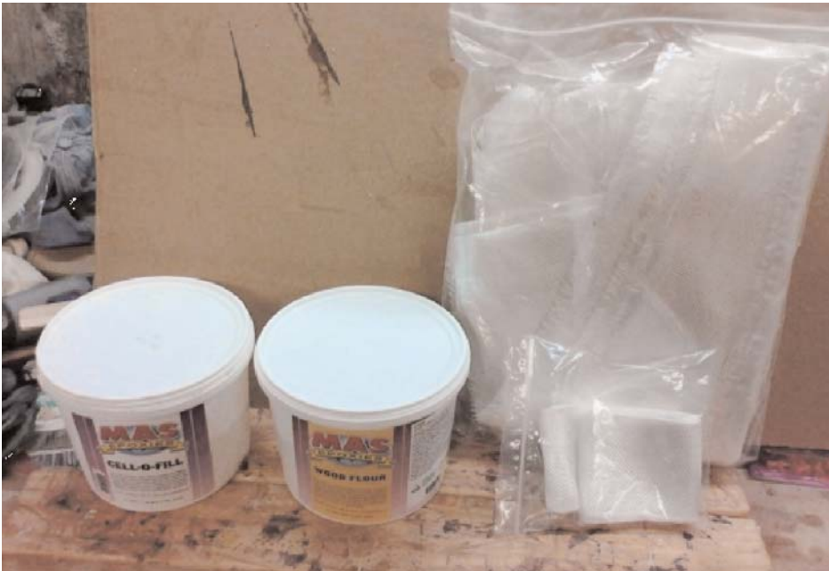
Containers of wood flour and cellulose are depicted. Fiberglass cloth and tape are also displayed.
