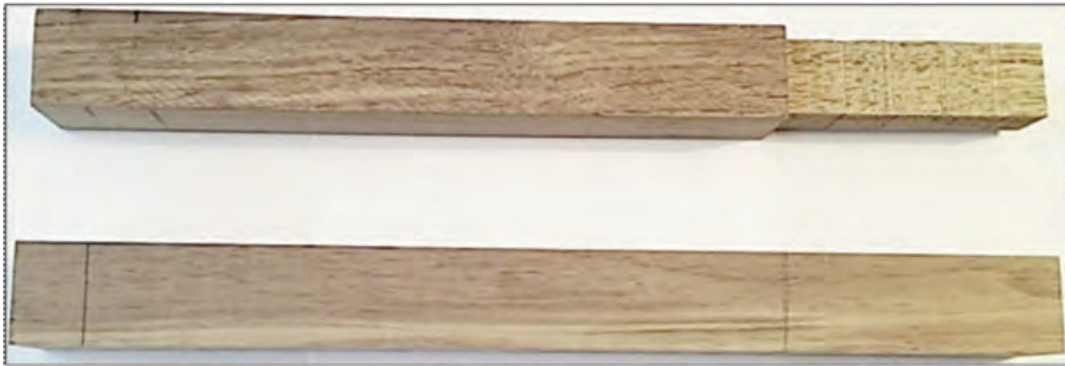
A rough-cut handle top section trimmed to final dimensions of 3/4" X 7/8" X 3 1/4"
