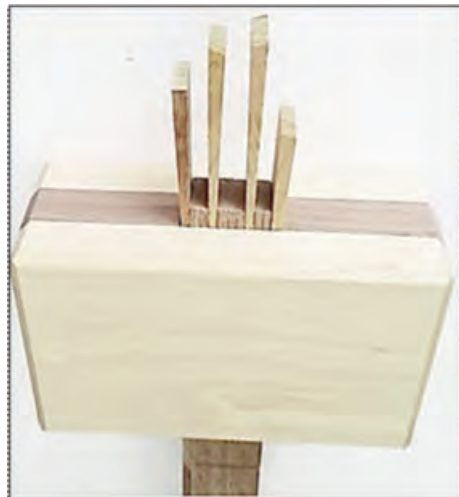
Shims started into the mallet head
