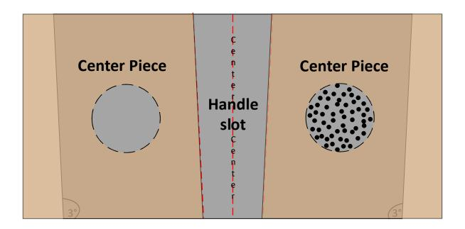
Add wood glue to the BBs. This prevents the BBs from rattling around when the mallet is in use. Allow 24 hours to dry.
