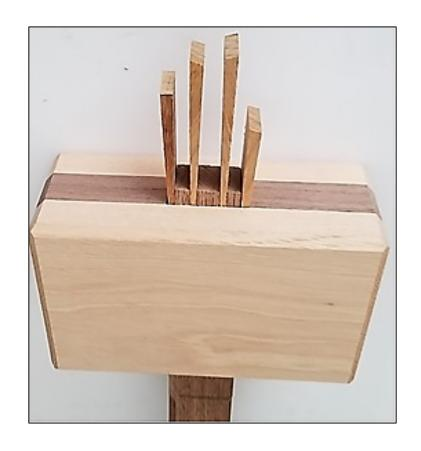
After the glue dries, use a flush-cut saw and remove protruding section; sand smooth.
