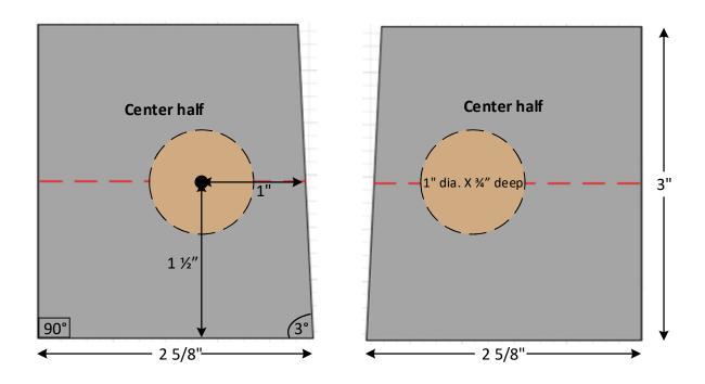
**Tip:** Drill holes before assembling the mallet head
